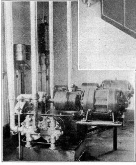
Top — Electro-pneumatic machine in tower
